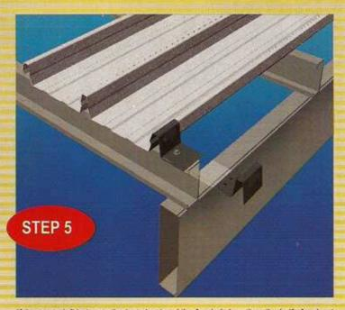
If the space left between the last sheet and the fascia is less than the half of a sheet width, it will be covered by the fascia capping. In this case, cut fastening clips to two and using the short leg half, secure the male rib at each purlin.
