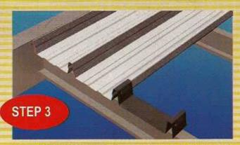
Position the short leg of the fastening clip over the male rib of the fastened sheet and, using appropriate fasteners secure the clip to the purlin.
